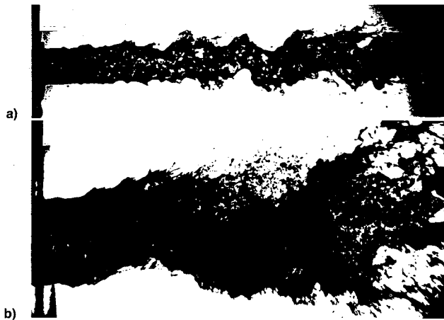
Fig. 16 Nonaxisymmetric oscillations of a liquid jet water/air: a) d_{jet} = 1 mm, u_f = 10 m/s, u_g = 50 m/s, p_g = 10 bar and b) d_{jet} = 2 mm, u_f = 3 m/s, u_g = 150 m/s, p_g = 1 bar.
