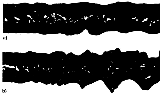
Fig. 11 Segment of a free liquid jet, Re_l = 10^4 : a) without coaxial gas and b) with coaxial gas: u_{\text{rel}} = 100 m/s.
